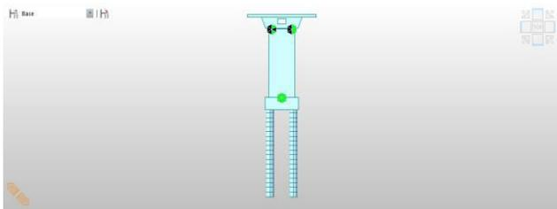
Fig.(5): Bridge POT PTFE bearing support cross section view
