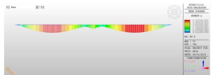
Fig. (2): Response spectra in x direction –BM in box Girder
