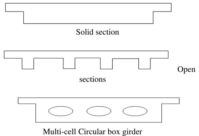
Fig (1): Various cross section of box girder
