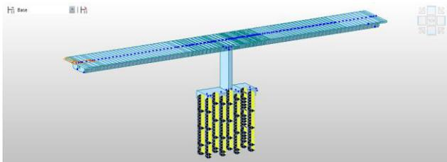
Fig.(6): Elastic spring for pile foundation
